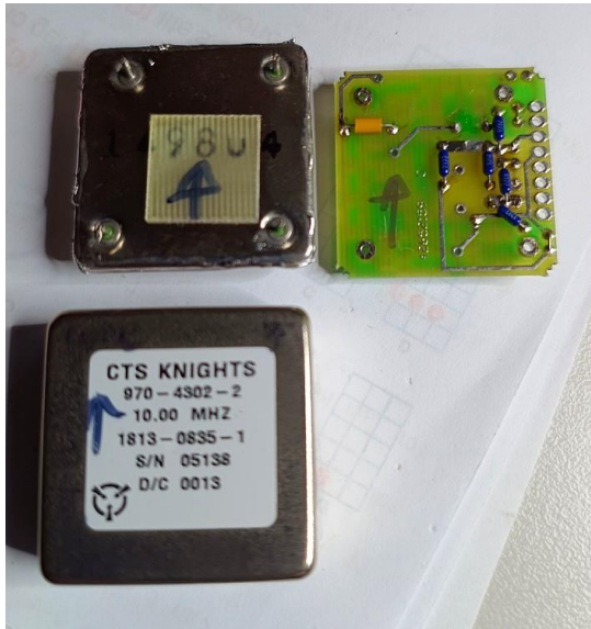
TCXO split apart - with guide arrows to help later on with re-assembly.
